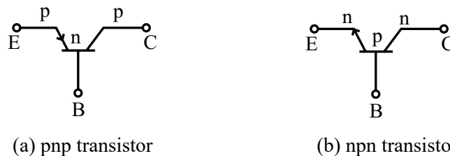
Fig. 2 Symbols of BJT (a) pnp transistor (b) npn transistor
